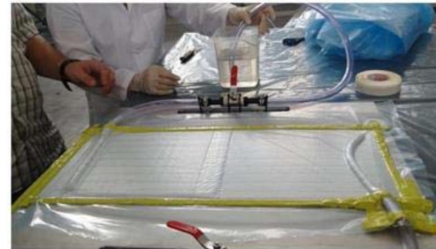
Resin infusion stacking
